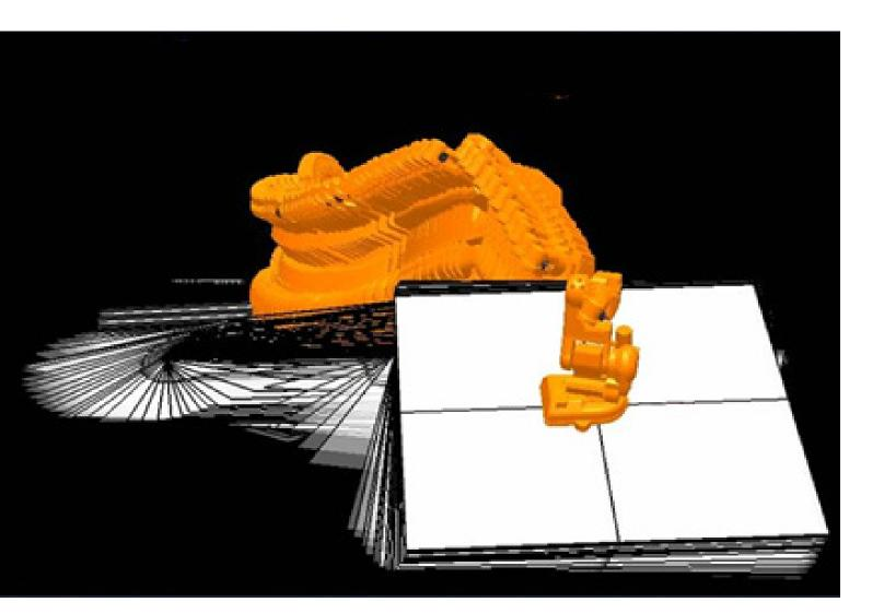
ABB's Robotics Division markets RobotStudio simulation and offl ine programming software, allowing robot programming to be done on a PC without shutting down production and increasing overall productivity.
