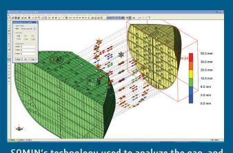
SAMIN's technology used to analyze the gap, and map the curved panel.
